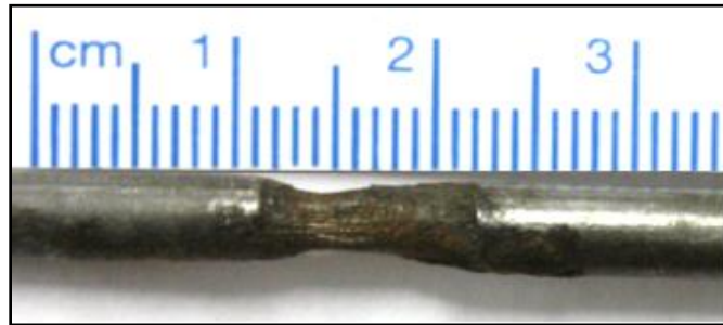
Figure 4.4 Observed corrosion influence zone and morphology at the intersection of preexisting crack with steel after demolishing at end of experiment. For the intersection indicated by the blue arrow in figure 4.3 (a)
