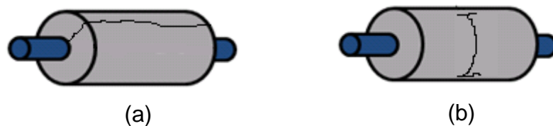
Figure 4.14 Illustration of observed orientations of induced cracking. (a) longitudinal and (b) circumferential, both across cylinder half, as a result of uniform and localized corrosion morphology along embedded rebar, respectively.
